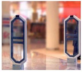
Magneto acoustic gate used for product surveillance
