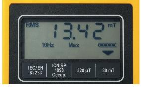
Broadband measurement in "mT" with RMS detector
