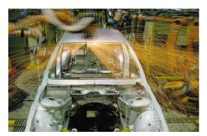
Resistance welding machinery in operation
