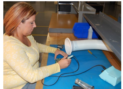
Two operators using the Floor Sentry Double units to extract soldering fumes simultaneously.
