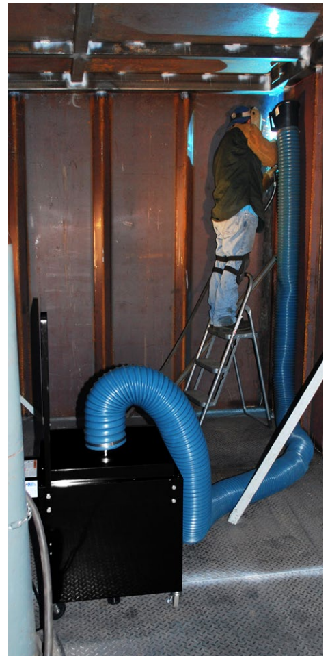
Python Portable Floor Sentry provides hands-free fume extraction for hard to reach areas and applications (SS-400-PYT pictured above)
