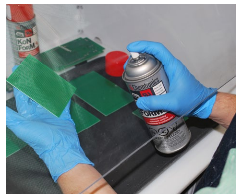
Closeup of operator safely spraying conformal coating under a DSH.
