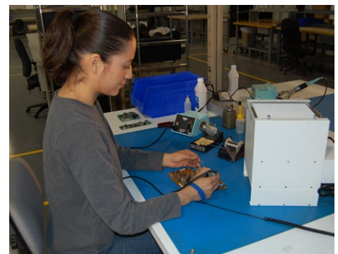
The operator is using the benchtop Model 200 Table Sentry to protect herself from inhaling harmful soldering fumes.
