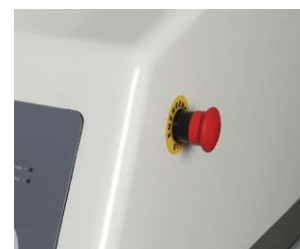
Emergency Stop for Operator Safety
