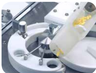
Patented radial transport rake
