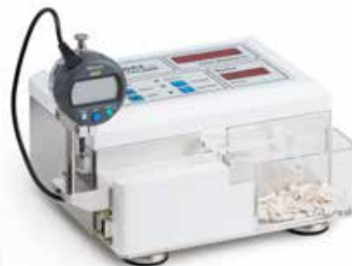
HC6.2 with external thickness gauge and scale
