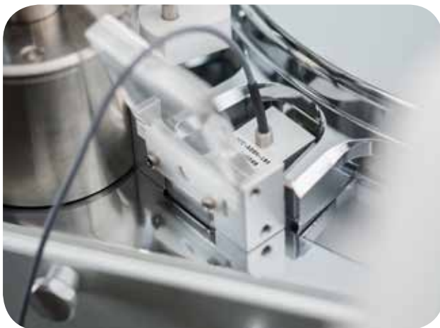
The load cell is placed in the breakage chamber of the tablet testing system to enable dynamic calibration
