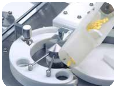
Patented radial transport rake
