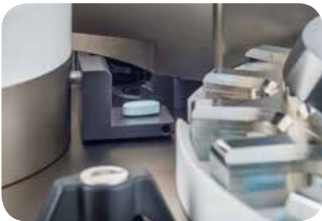
Precise tablet positioning (patented stamp)
