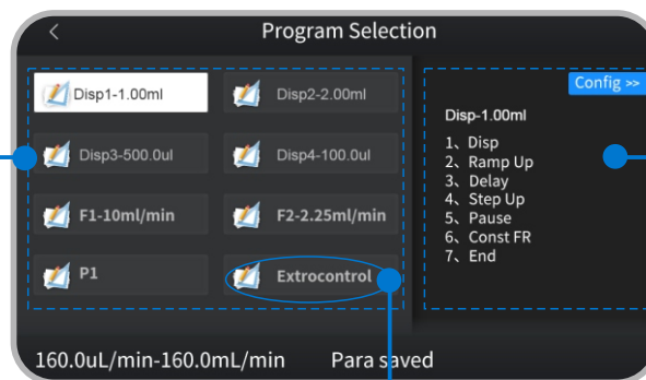
Preset external control program for remote control through external signal
