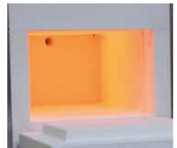
Muffle heated from four sides
