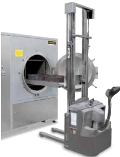
Charging of the retort furnace NRA 300/06 with a pallet truck
