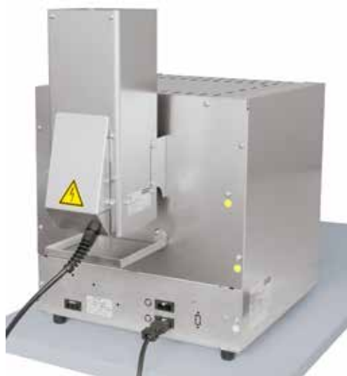
Standard laboratory muffle furnace L 5/11 with catalyst KAT 50 see page 14
