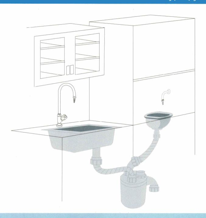
The one piece moulded Polypropylene Dilution Recovery Trap with a 4.5 litre capacity is Ideal for fumecupboard and underbench installations serving one or multiple sink. Its physical and high chemical resistant properties are well suited to dilute acid that poured into the sink. The process of dilution is important in the laboratory environment as it render the acid less harmful.
