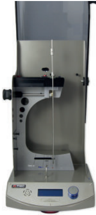
The gas-spring supported transparent draft cover allows easy access to all parts.
