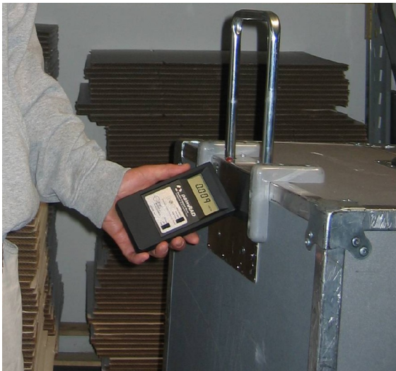
palmRAD 907 (shown left) being used to locate radiation and measure in \mu\text{R} .
