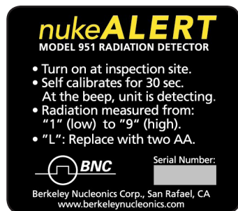
All display symbols are defined on the rear panel of the instrument, eliminating the need to carry a user manual.
